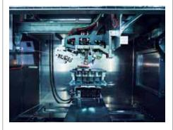
**B** oeing has recently signed an agreement with Norway's Norsk Titanium for additive production of titanium parts for the 787 Dreamliner, according to a statement from Norsk Titanium. According to a representative of the Norwegian manufacturer, additive technology, commonly called 3D printing, could help
