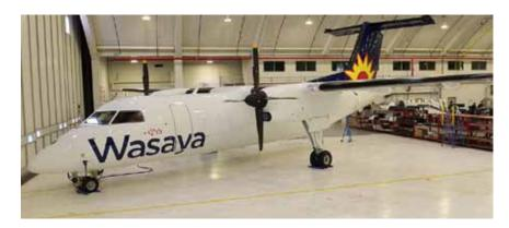
anadian aerospace company, Voyageur Aviation Corp. rolled out the first-of-its-kind Dash 8-100 Package Freighter (PF) conversion aircraft. The Dash 8-100 PF carries an average payload of 4.5 tonnes, and has 39 cubic meters of cargo space. The aircraft's 1.27-meter x 1.52-meter cargo door, and low door sill height of 1.02 meters, facilitates loading without specialized equipment. The aircraft is also equipped with a reinforced cargo floor and an advanced LED interior lighting system.
